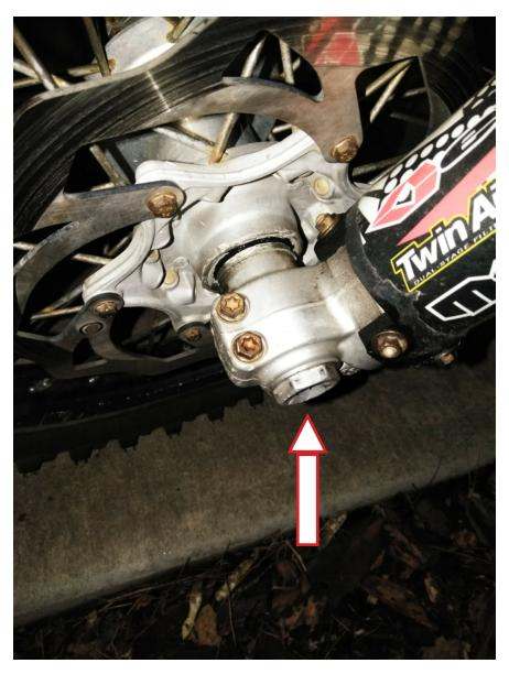
Tighten the front wheel axle to an initial torque value. The 2009 KTM 450 XC-W is 33.2 lb.ft using the 27mm socket. The 2000-2007 DRZ 400s is 14.5 lb.ft. using the 24mm socket on one end while holding the other end with the 19mm hex tool. The KX450F is 58 lb.ft. with a 22mm socket.
