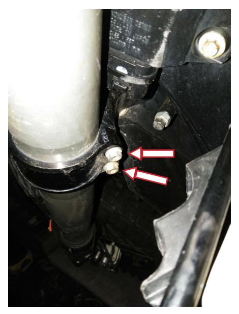
Tighten the four bolts (2 on each fork) of the lower triple clamp back up. The 2009 KTM 450 XC-W torque value is 8.9 lb.ft and socket size is 10mm. The 2000-2007 DRZ 400s torque value is 23.0 lb.ft. and socket size is 12mm. The 2011 KX450F torque is 15 lb.ft. and socket size iz 12mm.
