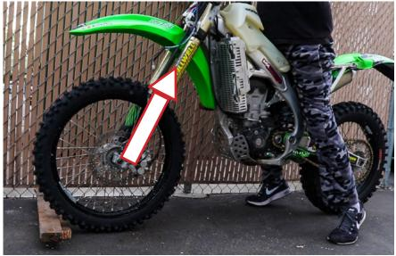
Block the front wheel and bounce the front end up and down 4 or 5 times WITHOUT holding the brake. This is what allows the front wheel to find its natural centered position.
