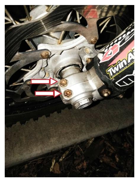
Loosen the four bolts clamping the axle to the forks (2 on each fork). 10mm socket for KTM. 12mm socket for DRZ and KX450F.
