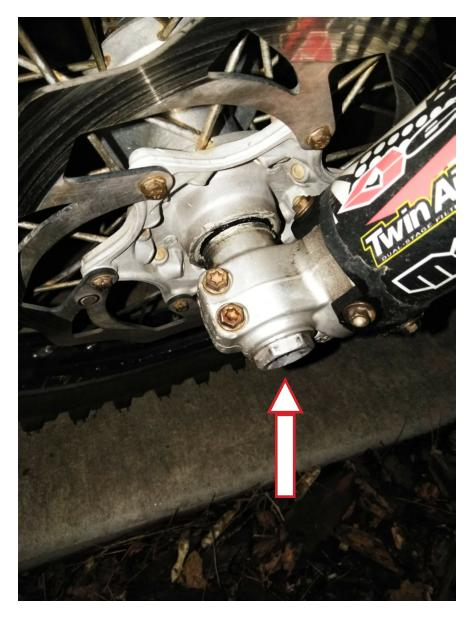
Loosen the front wheel axle nut. 27mm socket for KTM. DRZ uses 24mm socket on one end and 19mm hex tool on the other end. 2011 KX450F uses a 22mm socket and a 19mm hex tool.
