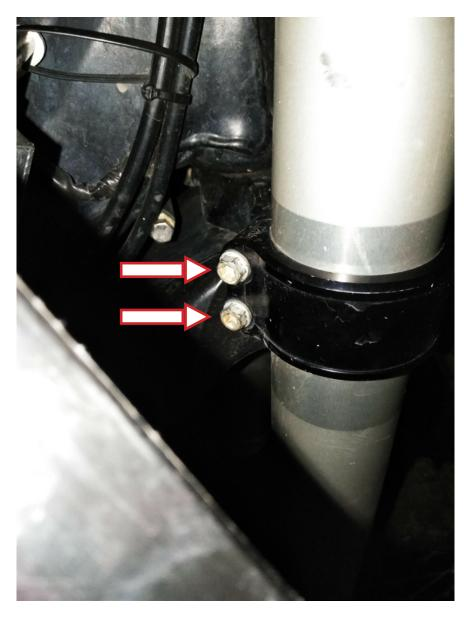
Loosen the four bolts (2 on each fork) holding the forks in the LOWER triple clamp. (2 bolts on each fork). 10mm socket for KTM. 12mm socket for DRZ and KX450F.
