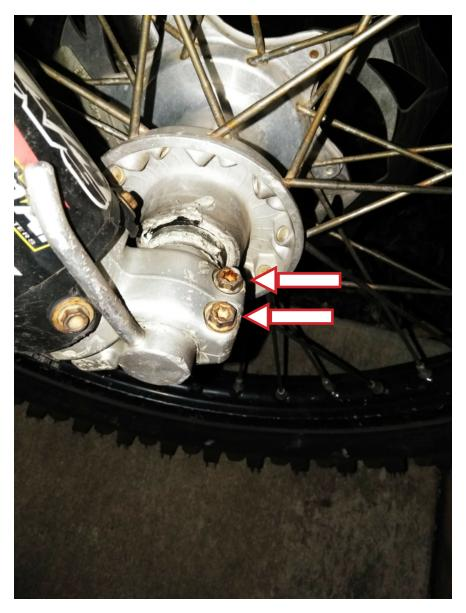
Tighten the four axle clamp bolts (2 on each fork). The 2009 KTM 450 XC-W torque value is 11.1 lb.ft. and socket size is 10mm. The 2000-2007 DRZ 400s torque value is 13.0 lb.ft.and socket size is 12mm. The 2011 KX450f torque is 15 lb.ft. with a 12mm socket.
