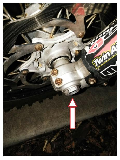
Tighten the front axle nut again to a final torque value. 2000-2007 DRZ 400s torque value is 30.5 lb.ft. using a 24mm socket.
