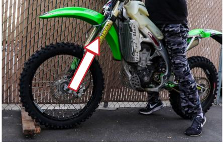
Bounce the front end up and down AGAIN. Do this 4 or 5 times by compressing the shocks with the front wheel blocked.
