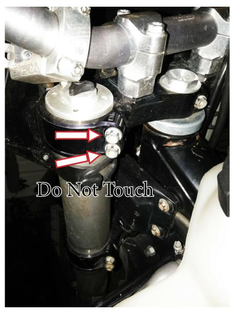
DO NOT loosen the top triple clamp as this would result in the forks completely sliding up through the triple clamp assembly.
